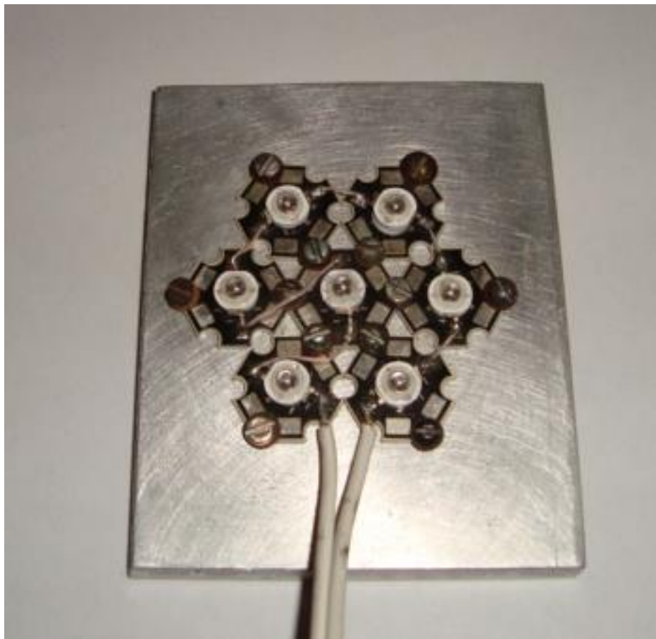
Figure 49. 60 watt power IR lighter.
