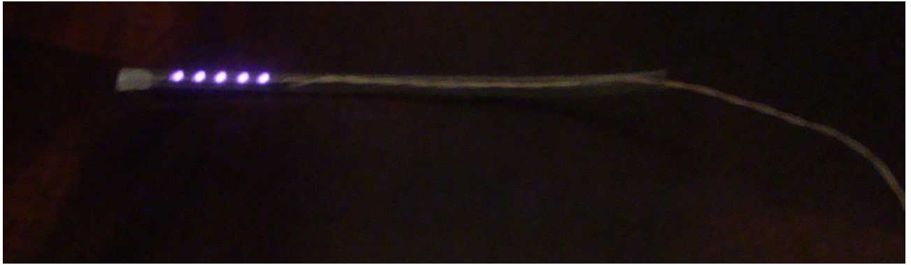
Figure 48. Urethral canal lighter device, composed of IR LEDs.
