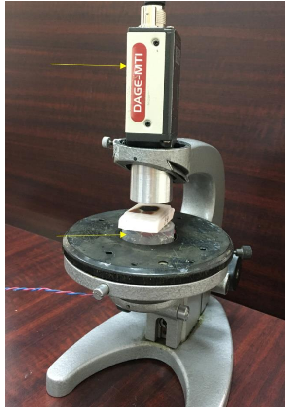
Figure 9. FFPE is placed between CCD camera. The LEDs (indicated by the arrow) are placed below the prostate tissue. The CCD camera, indicated by the arrow, is placed above the FFPE.
