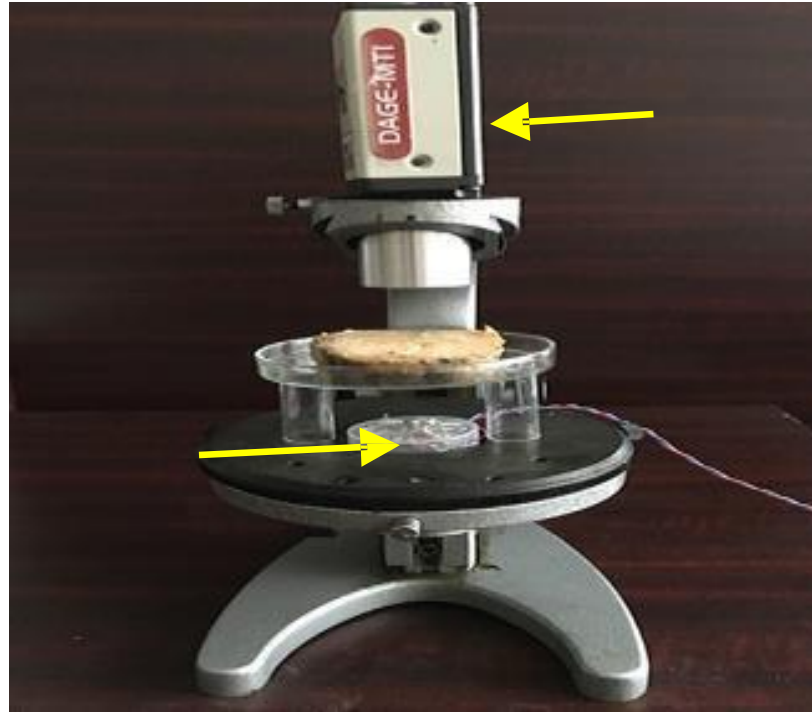
Figure 1. Experimental set up. Kidney specimen is placed on Petri dish. LEDs are placed under the specimen - shown with arrow. CCD camera (shown with arrow) is connected to PC. IR passing through kidney tissue carries information about optical density inhomogeneity caused by existence of cancerous formations.
