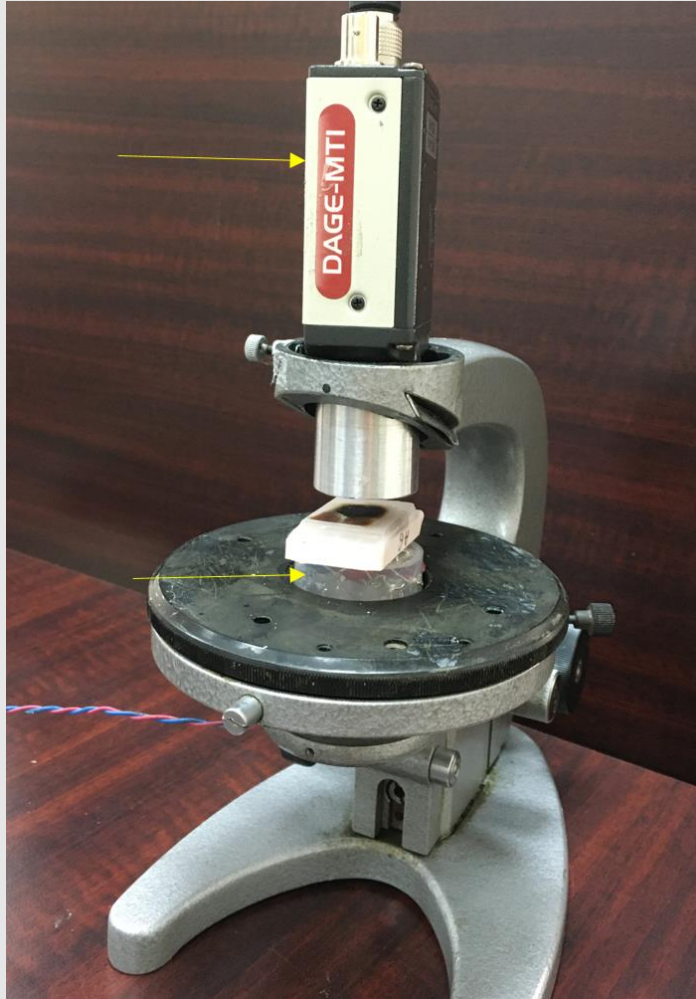
Figure 1. FFPE is placed between CCD camera. The LEDs (indicated by the arrow) are placed below the prostate tissue. The CCD camera, indicated by the arrow, is placed above the FFPE.
